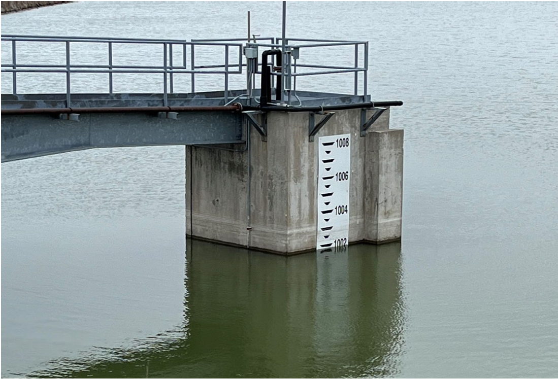
Photo 15 Pond 3 staff gauge, reading an elevation of 1001.8 feet (mean sea level). 11/11/2022
